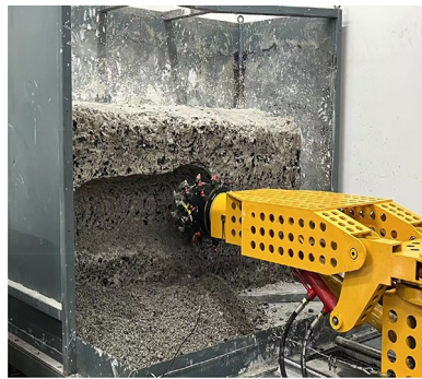
Figure 15. Test cutting process.
