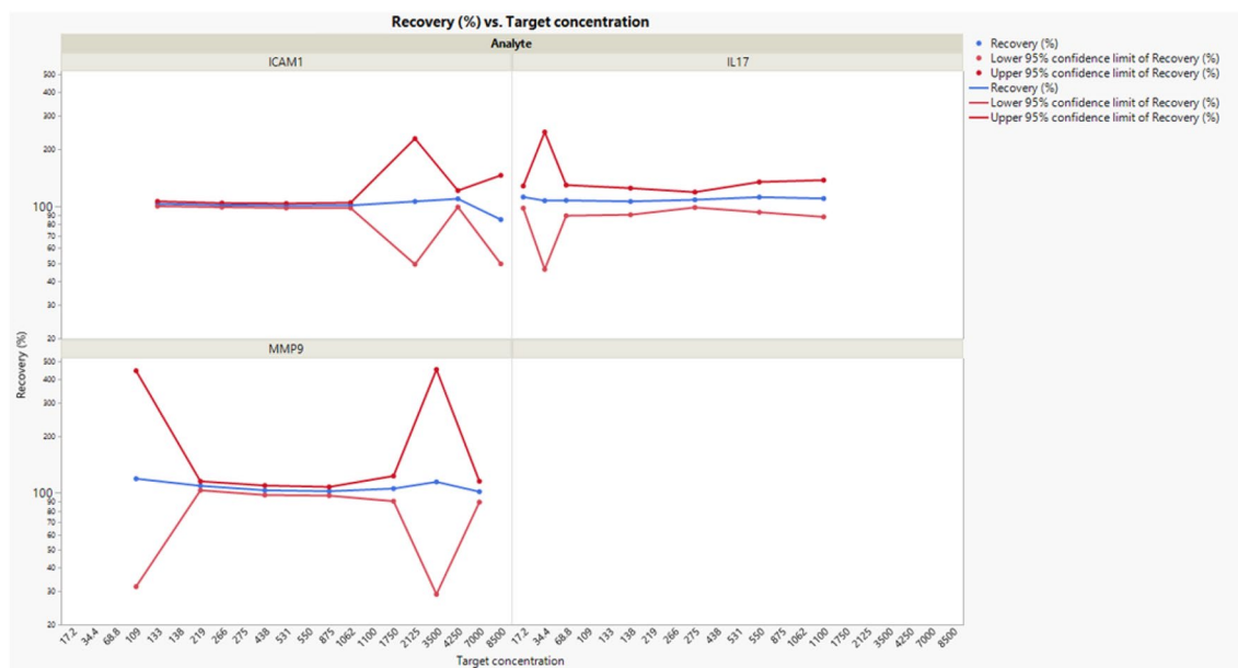
Figure 3. Trueness: evolution of recoveries (%) across concentration levels per analyte together with their corresponding 95% confidence intervals. Target concentrations are expressed in pg/ml. N=6 samples run in duplicates.
