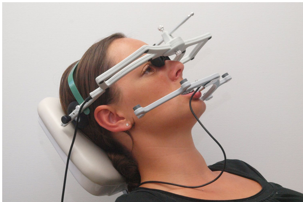
Figure 2. Example of a computer-aided motion recording system based on ultrasonic measurement technology (Zebris Jaw Motion Analyzer+, photo: Ahlers).
