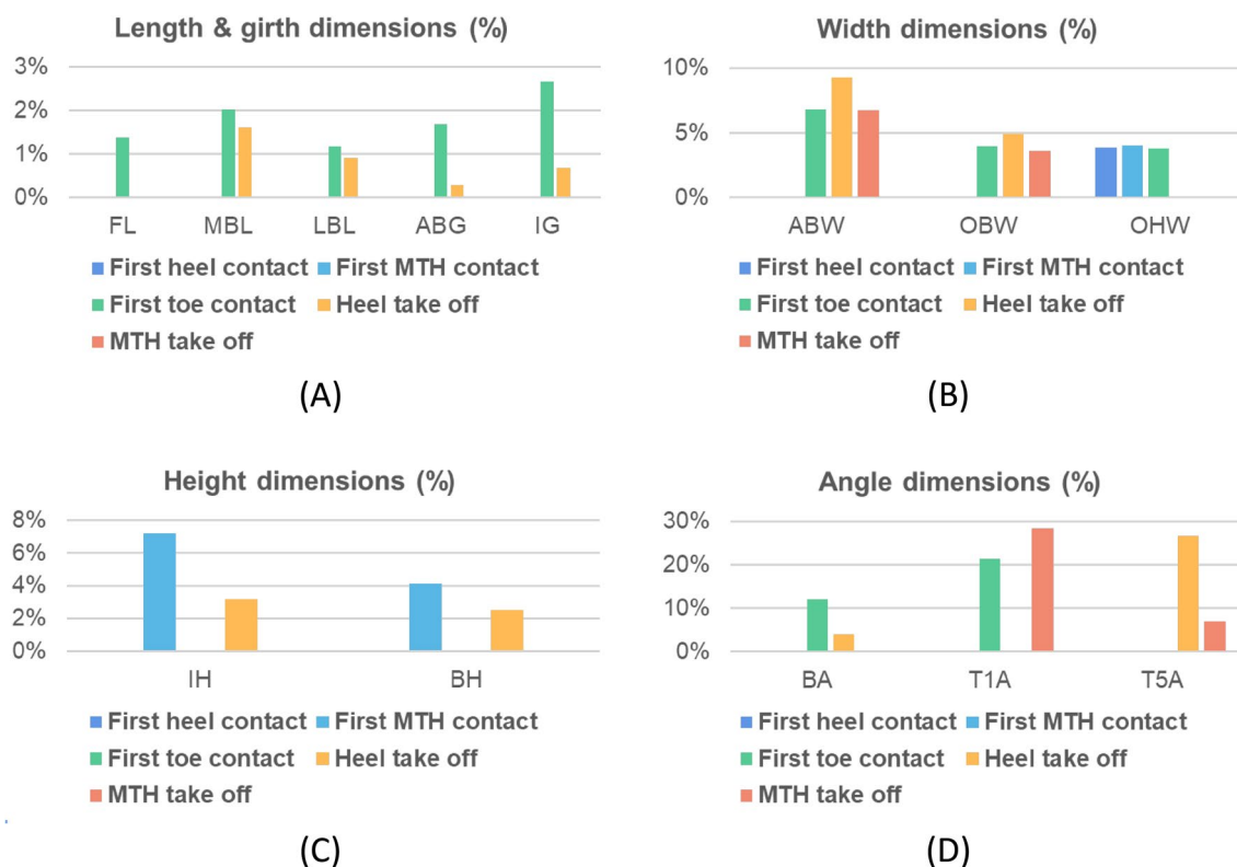
Figure 13. Change percentage of foot measurements during roll-over process: (A) length & girth dimensions; (B) width dimensions; (C) height dimensions; and (D) angle dimensions.
