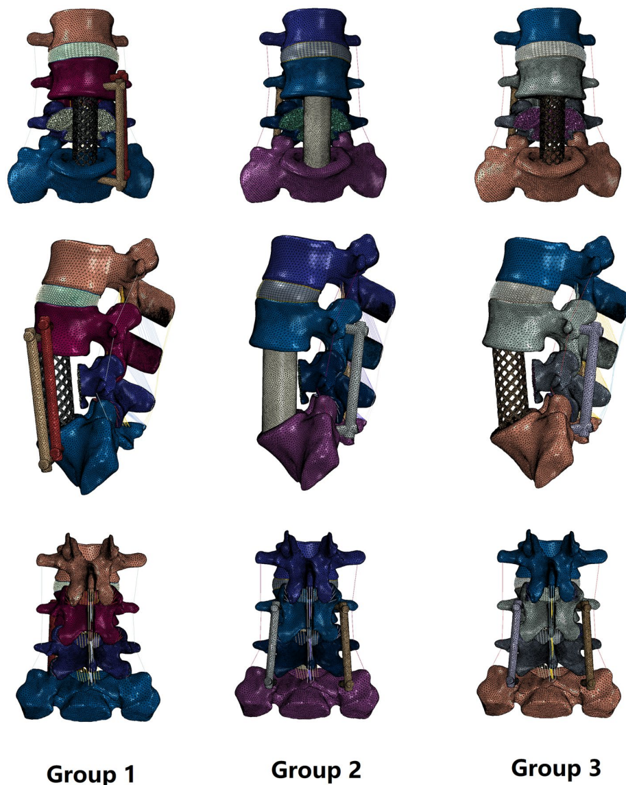
Figure 2. FE models of three lumbar internal fixation methods. Group 1-titanium cage combined with lateral double screw-rods fixation; Group 2-autologous bone combined with posterior double screw-rod fixation; Group 3-titanium cage combined with posterior double screw-rods fixation.
