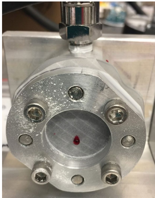
Figure 6. Picture of the dye penetration testing apparatus used after the partial puncture testing.
