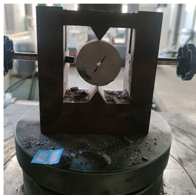
Figure 2. Disc shear loading method.
