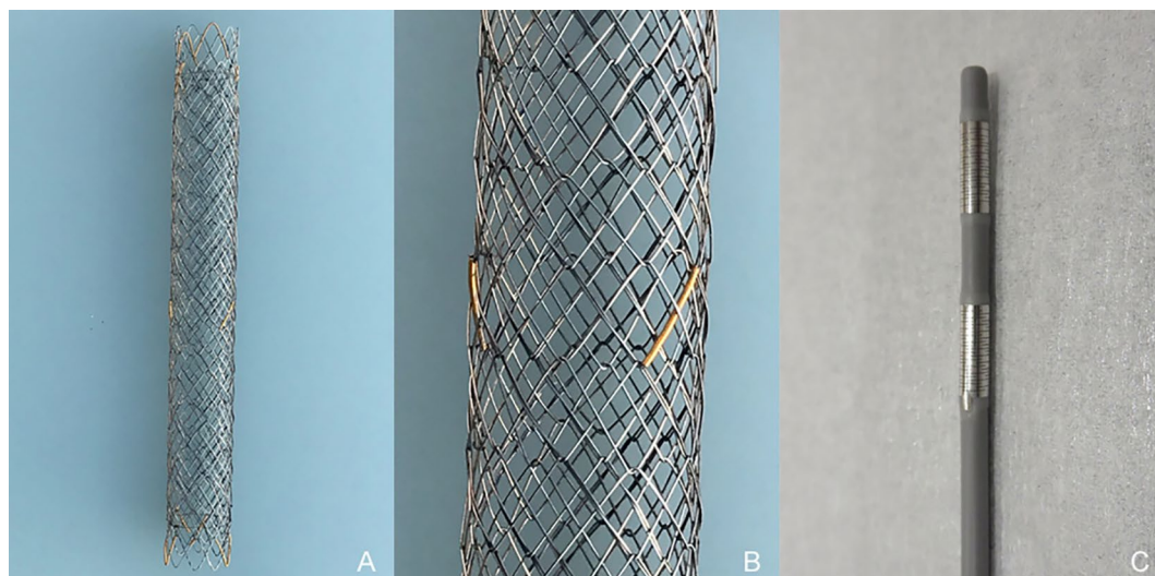
Figure 1. The structure of the EGIS biliary double bare stent (S&G Biotech, Seoul, Korea) is composed of two cross-overlapping standard uncovered stents, which can reduce the cell size and ensure sufficient radial force (A,B). The Habib EndoHPB catheter (Boston Scientific, Marlborough, MA, USA) is a bipolar catheter specializing in endobiliary radiofrequency ablation with two 8-mm ring electrodes placed 8-mm apart at the catheter tip (C).
