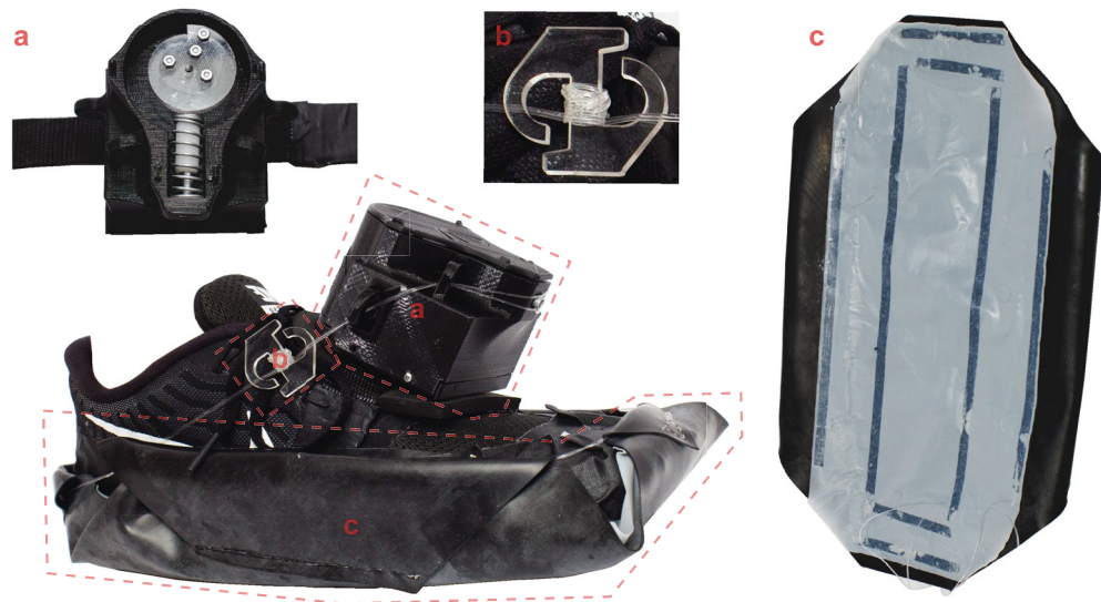
Figure 1. The Wearable Apparatus for Slip Perturbations (WASP) used in this study. This device consists of three components: (a) a wireless triggering mechanism consisting of a motorized cam-and-follower, (b) a tensioner that allows the device to fit securely to a range of shoe sizes, and (c) a flexible rubber outsole laminated with a polytetrafluoroethylene sheet that supplies both the friction with the ground to walk naturally in its attached state and the low-friction surface that participants are exposed to upon triggering. Lubricant was applied between the shoe and the outsole between each trial to further reduce friction upon outsole release.
