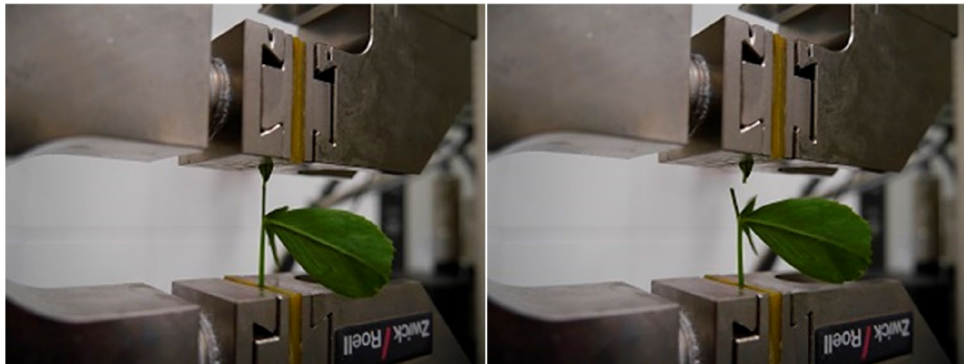
Figure 3. Before and after tensioning with the Zwick/Roell Z005 instrument. Photo by Agata Dziwulska-Hunek.
