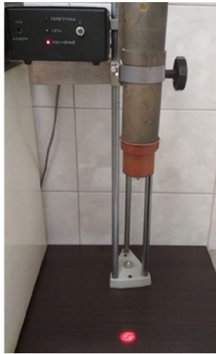
Figure 1. Self-designed rig for laser light stimulation of seeds. Photo by Agata Dziwulska-Hunek.
