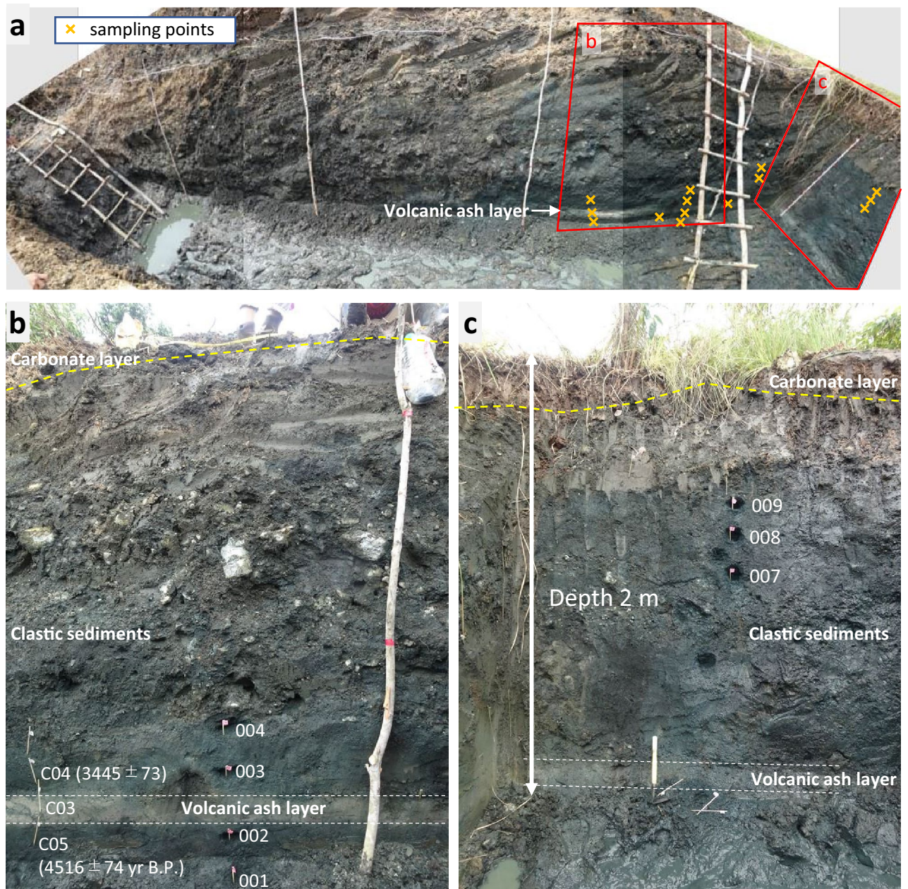
Figure 1. Outcrop photographs of the ultramafic clastic sediment containing a volcanic ash layer: (a) Overhead shot photograph of a trench where the crosses denote sampling points. (b,c) Cross-section of the trench. Solid samples were collected at different depth indicated by small flags. The numbers in parentheses are the ^{14}\text{C} ages of humin extracted from the clastic sediments (years before present).
