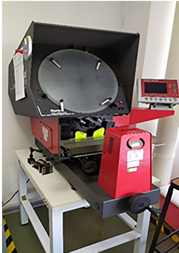
Figure 6. The profile projector (Starrett 400 SERIES).
