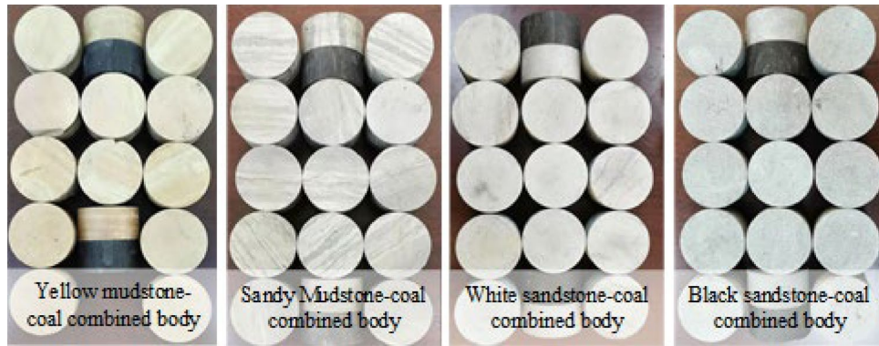
Figure 2. CRCB specimens prepared with four different rock sample and identical coal samples.
