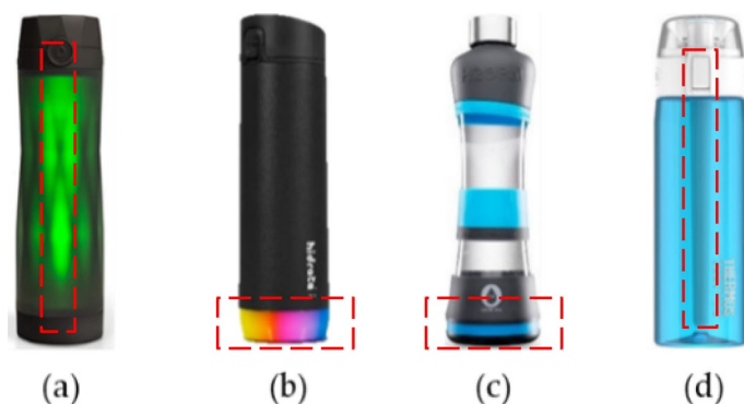
Figure 1. Images of analyzed commercial bottles: (a) HidrateSpark 3 4 , (b) HidrateSpark Steel 5 , (c) H2OPal 6 , (d) Thermos Smart Lid 7 . The dashed red boxes show the location of the sensors.
