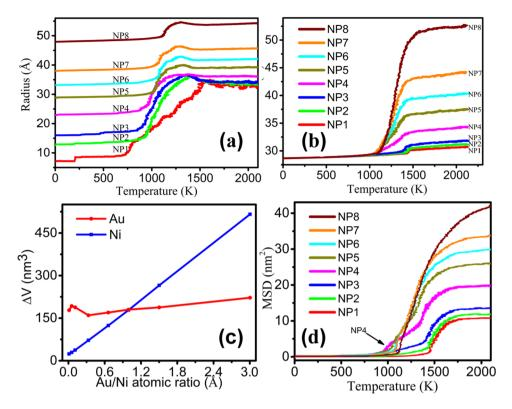
**Figure 6.** Evolution of radius of Au atoms (**a**) and Ni atoms (**b**) during heating process, (**c**) Volume change versus Au/Ni atomic ratio (**d**) MSD of NP1-NP8.
