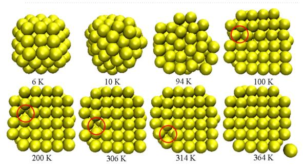
**Figure 3.** Snapshots of cross sections of Au atoms in the Au-Ni bimetallic NPs taken at eight representative temperatures (unchanged of (100) face of Ni atoms, as shown in the Fig. 2c).
