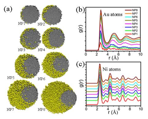
**Figure 5.** (a) Cross sections through the Au-Ni NPs at temperature 1173 K. (b,c) PDF of Au atoms and Ni atoms at temperatures 1173 K, Au and Ni atoms are colored in yellow and gray respectively.
