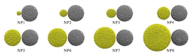
**Figure 1.** Initial configurations of Ni-Au NPs structures with different atomic ratio, Au and Ni atoms are colored in yellow and gray, respectively.
