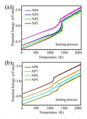
**Figure 4.** Variation of potential energy as function of temperature for the NPs heating process (**a**) NP1, NP2, NP3, NP4 (**b**) NP5, NP6, NP7, NP8.
