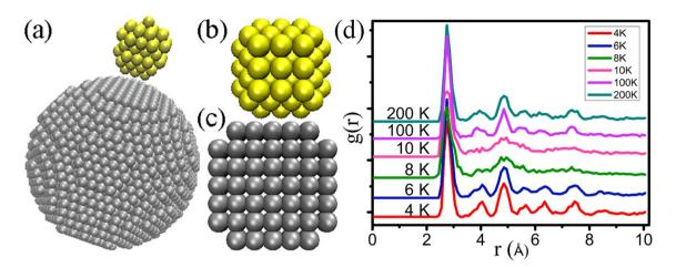
**Figure 2.** (a) The configurations of the simulated NP1 after a relaxation (b) (100) face of Au atoms (c) (100) face of Ni atoms (d) PDF of Au atoms in various temperatures.
