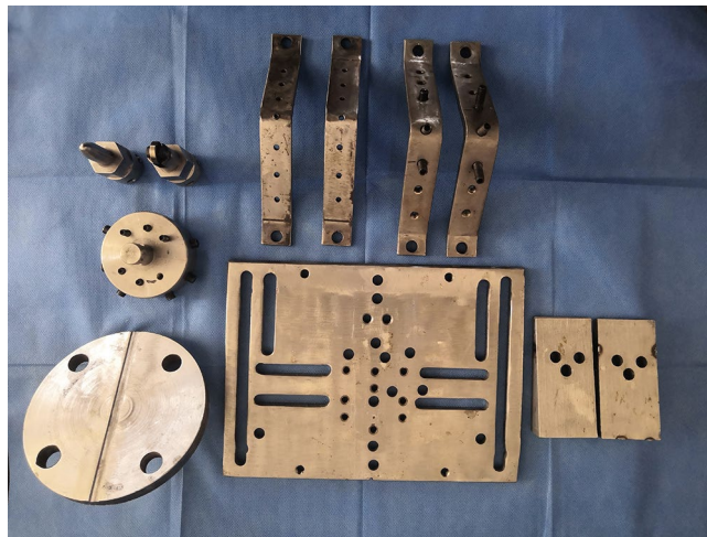
Figure 12. The special designed fixture for both fixing calf spine model and connecting with the testing machine.
