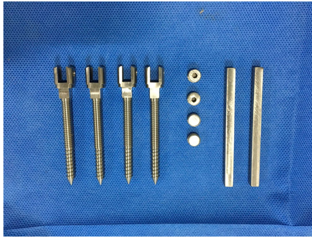
Figure 11. The special designed screws (diameter = 6.5 mm) and connecting rods (side length = 5.5 mm) for attaching strain gauges.
