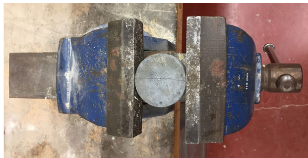
Figure 2. Cracking of mortar specimens using screw jack.
