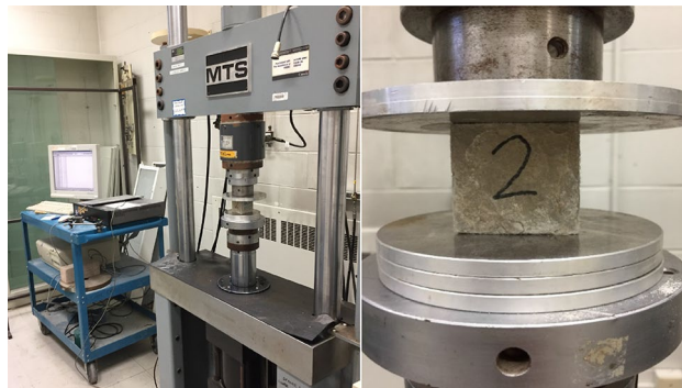
Figure 1. Cracking of mortar specimens using MTS machine.
