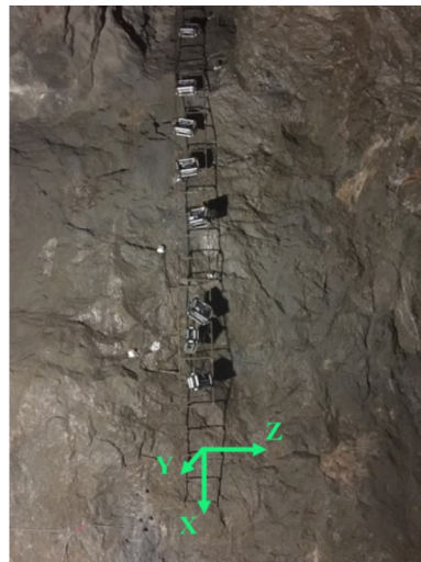
Figure 3. Installation drawing for site survey points.
