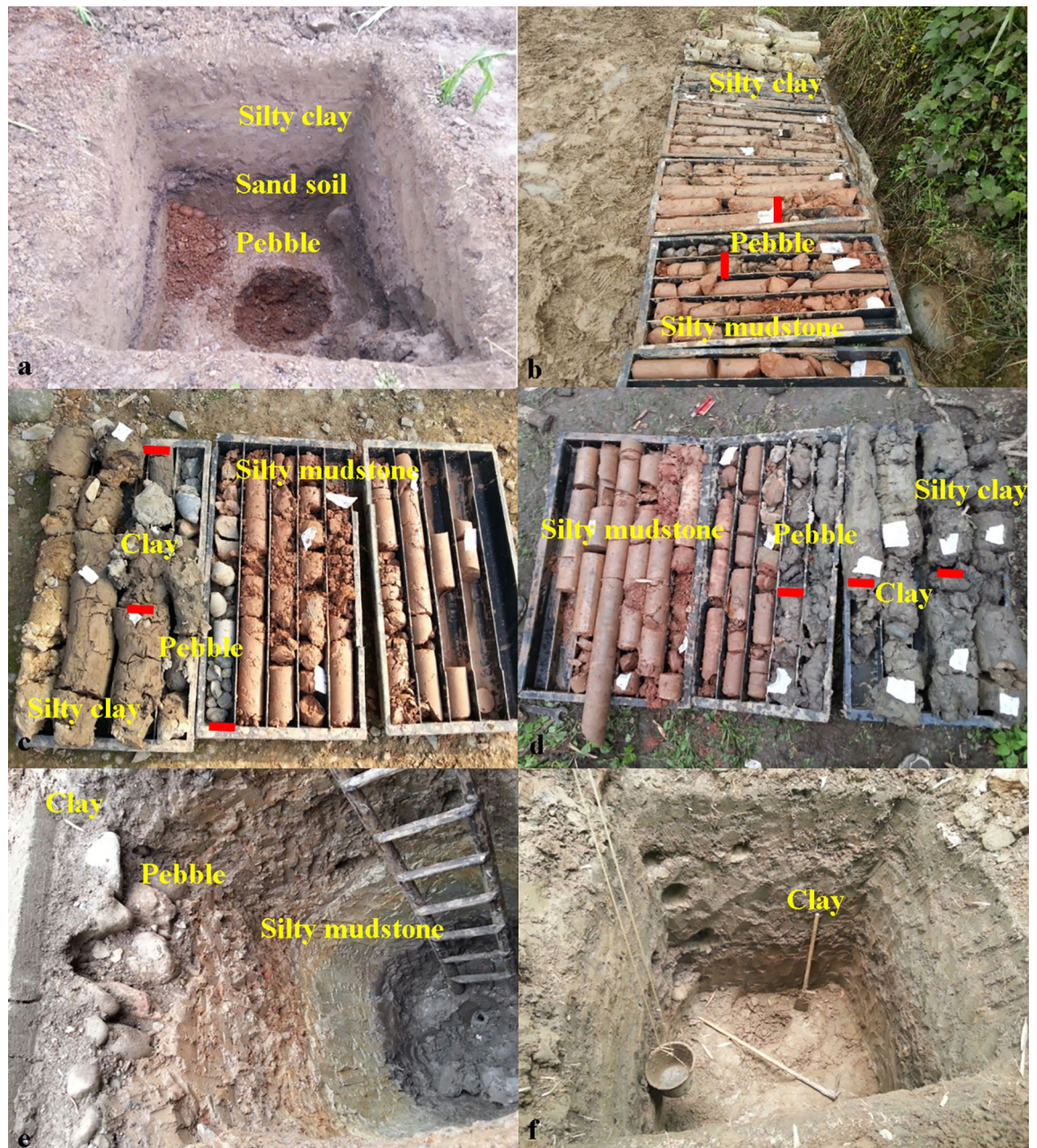
Figure 6. Lithological stratigraphic logs of boreholes and exploratory trenches. (a) TC-9. (b) B03. (c) B05. (d) B06. (e) TC-4. (f) TC-7.
