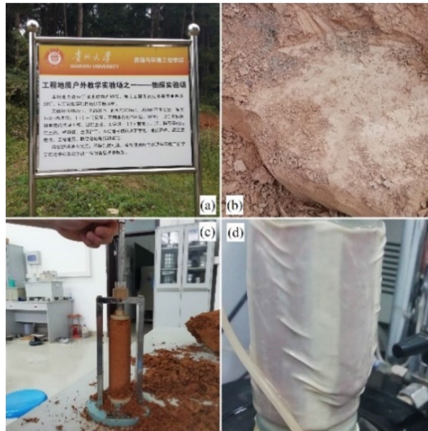
Figure 1. The appearance characteristics of land points and test sample 34 . (a) Land points; (b) field soil samples; (c) test sample; (d) soil sample in experiment.
