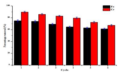
Figure 19. Effect of regeneration cycles on the percentage removal efficiency of Fe and Cr onto kaolin.
