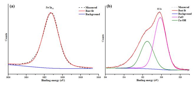
**Figure 9.** XPS profiles of ZnO nanoparticles for (**a**) Zn and (**b**) O 1*s*.
