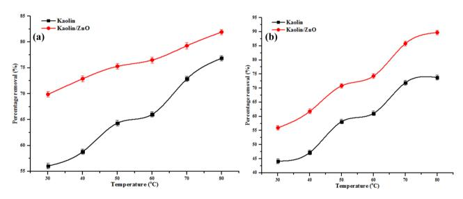
**Figure 17.** Effect of temperature on (**a**) Cr and (**b**) Fe ion removal onto kaolin and kaolin/ZnO (adsorbent dosage, 0.2 g, contact time, 15 min, agitation speed 150 rpm and pH 5.84). Errors bars signify means ± standard errors from the mean of duplicate experiments.
