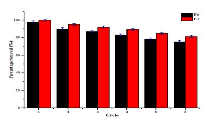
**Figure 20.** Effect of regeneration cycles on the percentage removal efficiency of Fe and Cr onto kaolin/ZnO nanoadsorbents.
