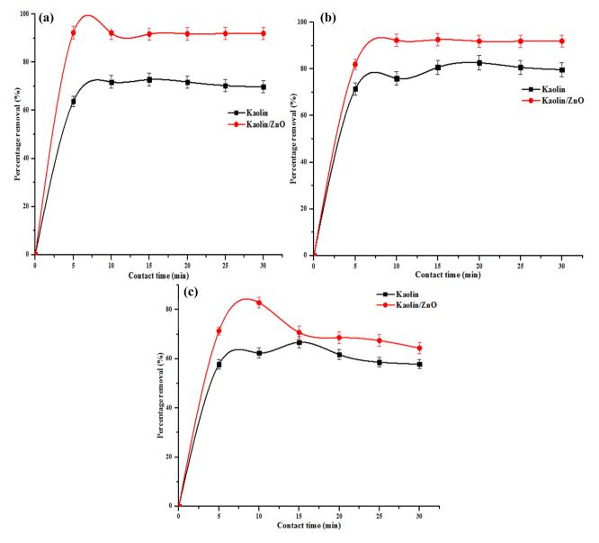
**Figure 12.** Effect of contact time on (**a**) COD (**b**) BOD and (**c**) chloride removal onto kaolin and kaolin/ ZnO (adsorbent dose 0.2 g, agitation speed 150 rpm, temperature 29 °C and pH 5.84). Errors bars signify means ± standard errors from the mean of duplicate experiments.
