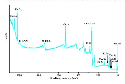
Figure 10. XPS general survey spectra of ZnO/kaolin nanocomposites.
