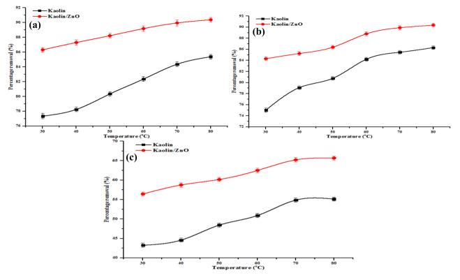
**Figure 16.** Effect of temperature on (**a**) COD, (**b**) BOD and (**c**) chloride removal onto kaolin and kaolin/ ZnO (adsorbent dosage, 0.2 g, contact time, 15 min, agitation speed 150 rpm and pH 5.84). Errors bars signify means ± standard errors from the mean of duplicate experiments.
