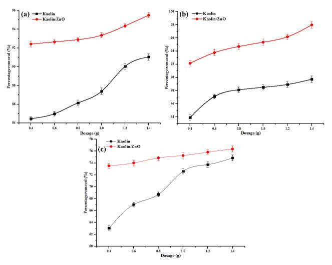
**Figure 14.** Effect of dosage on (**a**) COD, (**b**) BOD and (**c**) chloride removal onto kaolin and kaolin/ ZnO (agitation speed 150 rpm, contact time, 15 min, temperature 29 °C and pH 5.84). Errors bars signify means ± standard errors from the mean of duplicate experiments.
