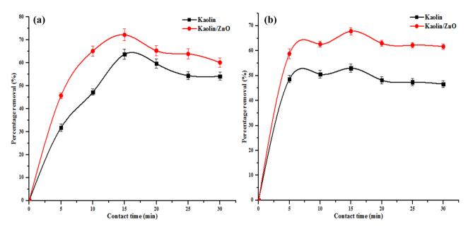
**Figure 13.** Effect of contact time on (**a**) Cr and (**b**) Fe ions removal onto kaolin and kaolin/ZnO (adsorbent dose 0.2 g, agitation speed 150 rpm, temperature 29 °C and pH 5.84). Errors bars signify means ± standard errors from the mean of duplicate experiments.
