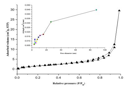
**Figure 7.** BET analysis for pore diameter (inlet) and surface area of kaolin/ZnO nanocomposites at a pH of 8.
