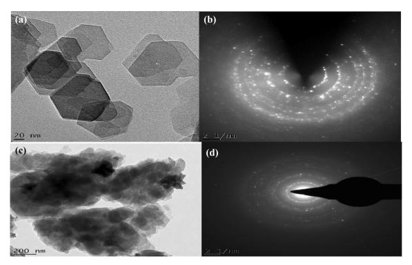
**Figure 4.** HRTEM and SAED analysis of beneficiated kaolin (**a**, **b**) and kaolin/ZnO (**c**, **d**) nanocomposites at pH of 8.
