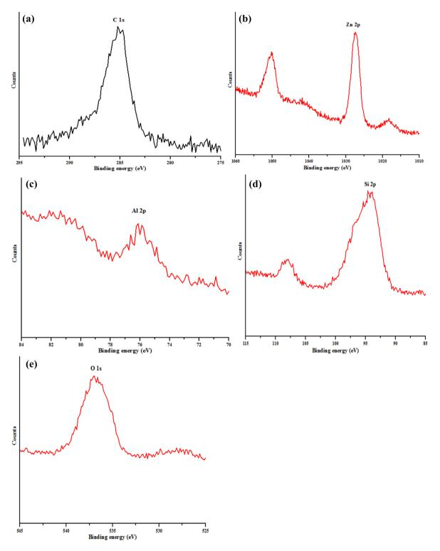
**Figure 11.** High resolution of XPS spectra of (a) C 1*s*, (b) Zn 2*p*, (c) Al 2*p*, (d) Si 2*p* and (*e*) O 1*s* for the synthesized ZnO/kaolin nanocomposites.
