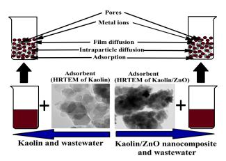
Figure 18. Steps in the adsorption mechanism.
