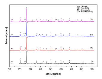
**Figure 2.** XRD pattern of kaolin/ZnO nanocomposites at pH (a) 6 (b) 8 (c) 10 and (d) 12 at calcination temperature of 450 °C for 3 h.
