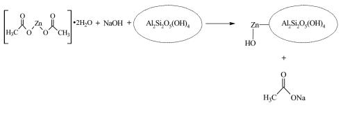
Figure 1. A schematic representation for preparation of kaolin/ZnO nanocomposites.
