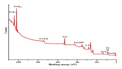
Figure 8. XPS general survey spectra of ZnO nanoparticles.
