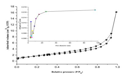
**Figure 6.** BET analysis for pore diameter (inlet) and surface area of kaolin.
