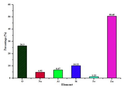
Figure 5. EDX analysis (atomic percentage) of kaolin/ZnO nanocomposites at a pH of 8.
