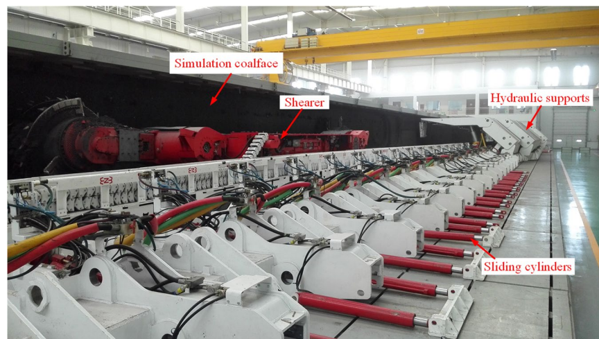
Figure 10. Test platform for shearer mechanical test.
