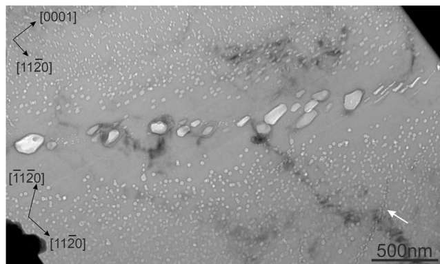
Figure 6. A high-angle GB with misorientation angle of \sim 90^\circ in a pebble irradiated at 713 K. Dislocation line decorated by Fe-Al-Be precipitates and gas bubbles is marked by arrow.
