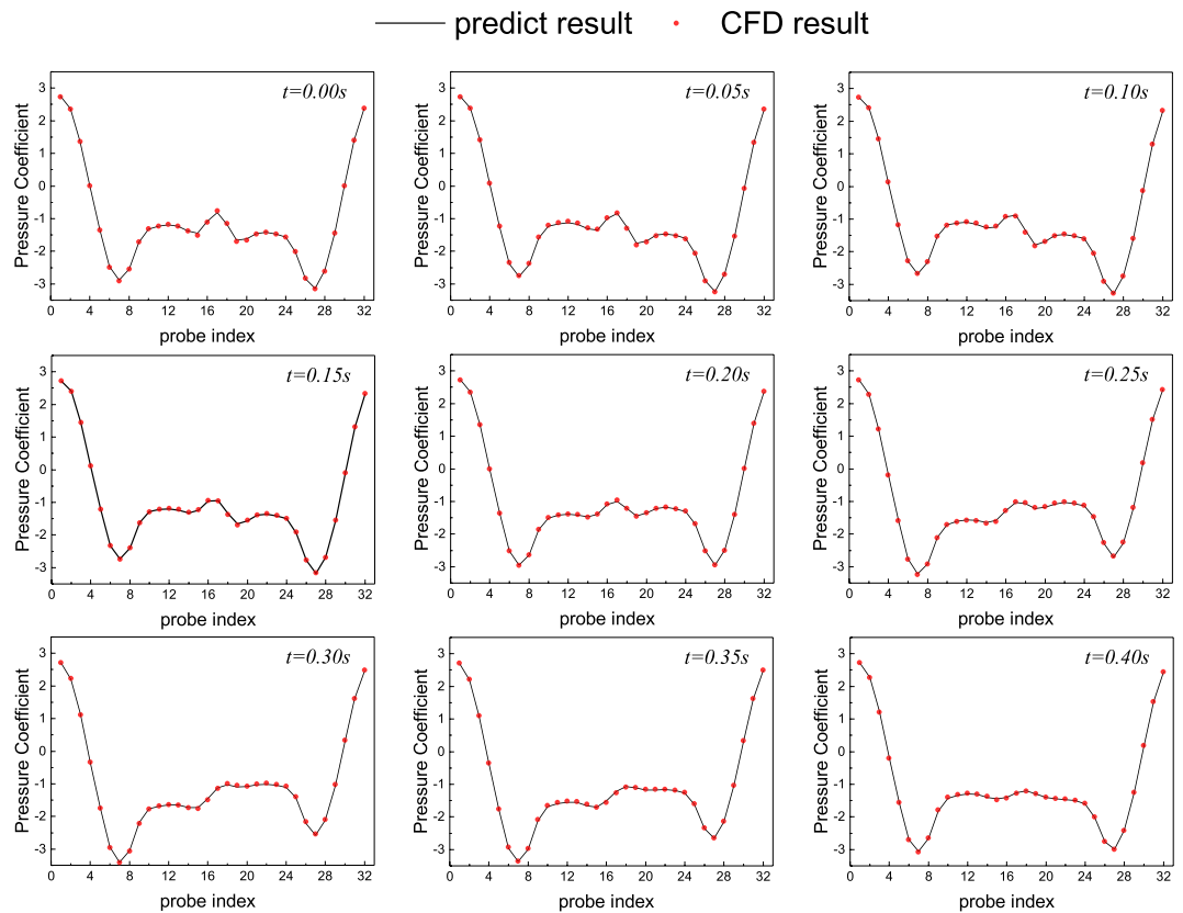
Figure 6. Comparisons of pressure coefficient on 32 points on the cylinder between the model predictions and CFD results with Reynolds number = 10000 at different moments. The red line is regarded as the standard result which we calculated in CFD method before, and the blue line stands for the predicted results through the CNN.
