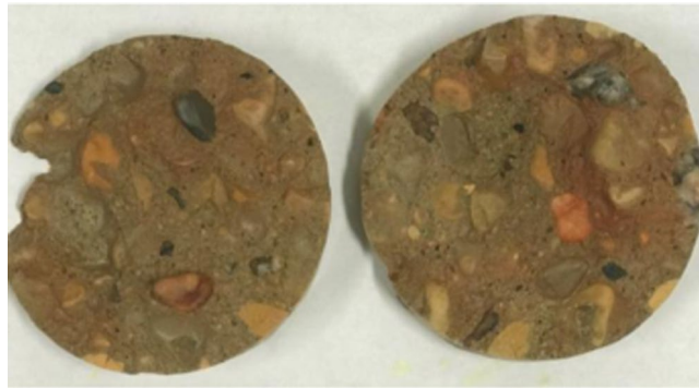
Figure 4. Concrete sample cut after saturating process with dyed DDW through GEIWIP test.
