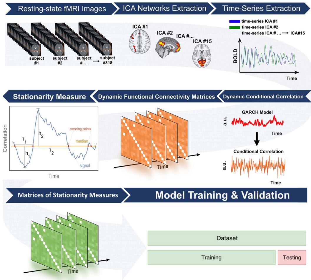
Figure 6. Image analysis workflow. The resting-state functional magnetic imaging (fMRI) data were initially pre-processed and next a set of 15 separate brain circuits were extracted via independent components analysis (ICA). Next, time-series from each ICA brain circuit were obtained from each individual and fed into dynamic conditional correlation (DCC) models. This led to 15 \times 15 time-variant functional connectivity matrices at the single-subject level that were then used to estimate non-stationarity “T”-index as in Zalesky et al. 27 . Finally, these “T”-index values were analyzed in conjunction with the traits of the five-factor-model of personality at the group level. The generalization ability of the model was evaluated using a train/test split approach (see the statistical analyses section of the methods for further information).
