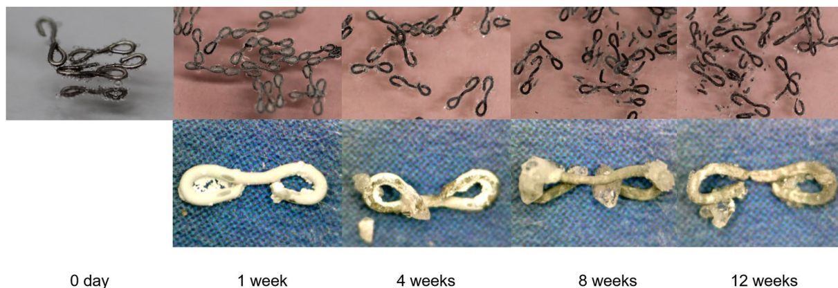
Figure 2. Immersion test using artificial intestinal juice. Macroscopic view of the developed Mg alloy staples at zero, one, four, eight, and 12 weeks after immersion (above) and Mg alloy staples removed after immersion (lower). The surfaces of the staples were covered with a layer of white corrosion product.
