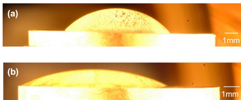
Figure 5. Horizontal view of drop shapes on platinum substrate at 1473 K under (a) Ar and (b) dry-air atmospheres.
