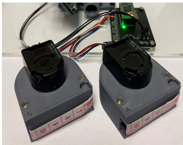
Fig. 3 Rotary encoder dynamic circumference tape measures 51 .
