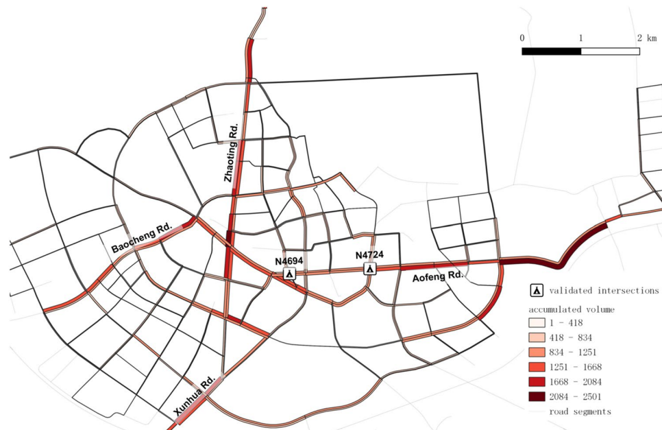
Fig. 7 Morning peak traffic in Xuancheng city. The width of the blue shades represents the number of vehicles. Road segments (Zhaoting, Baocheng, Xunhua, and Aofeng Rd.) and intersections (N4694 & N4724) are to be validated.
