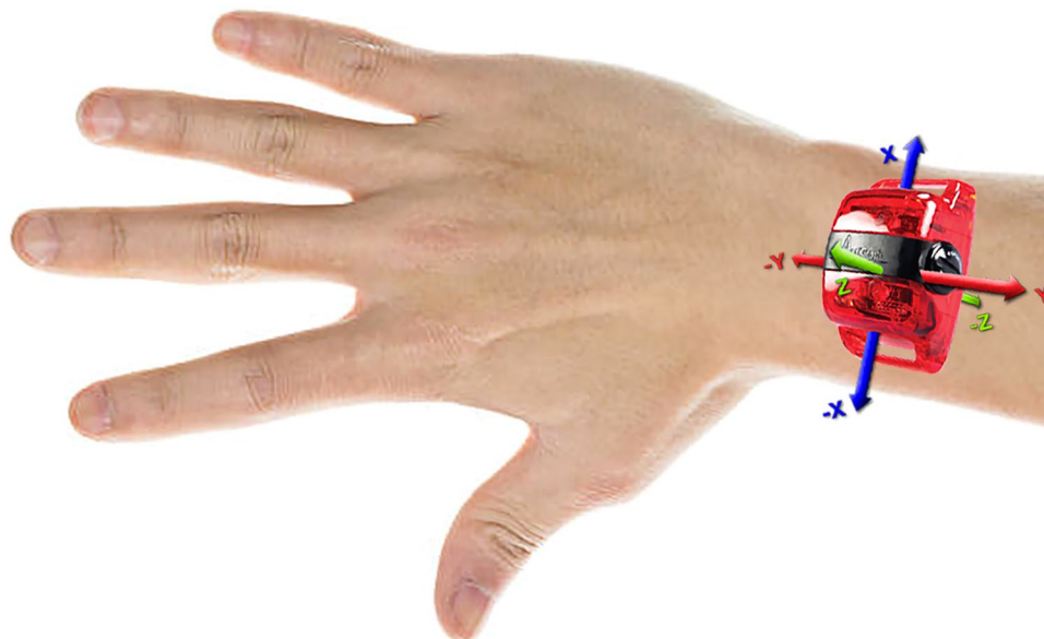
Fig. 2 Sensor orientation. Direction of the three acceleration axes (participants were instructed to wear the monitor on the back of the wrist with the + ve y axis pointing up the forearm away from the hand).
