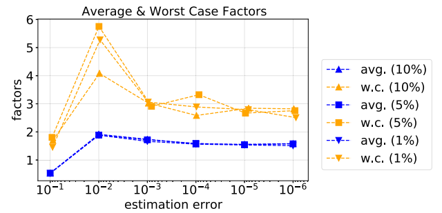
Fig. 4 Analysis of constant overhead for Chernoff-Hoeffding IQAE. The average (blue) and worst-case (orange) constant overhead for IQAE runs with different parameter settings.
