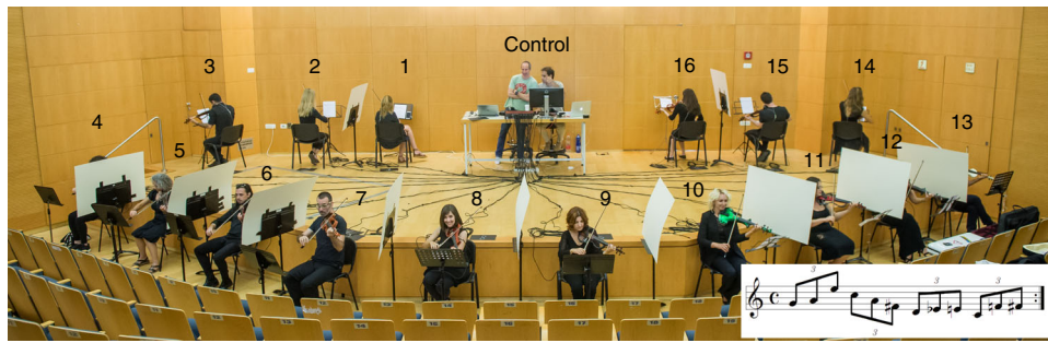
Fig. 1 Sixteen coupled electric violin players repeating a musical phrase. Sixteen violin players are playing with electric violins. The audio output from each violin is connected to our computer-controlled mixing system. Then, the mixing system sends to the headphones of each player a sum of audio signals of the desired connectivity, strength, and delay. All participants in the picture have approved publishing it. The musical phrase is presented in the inset.
