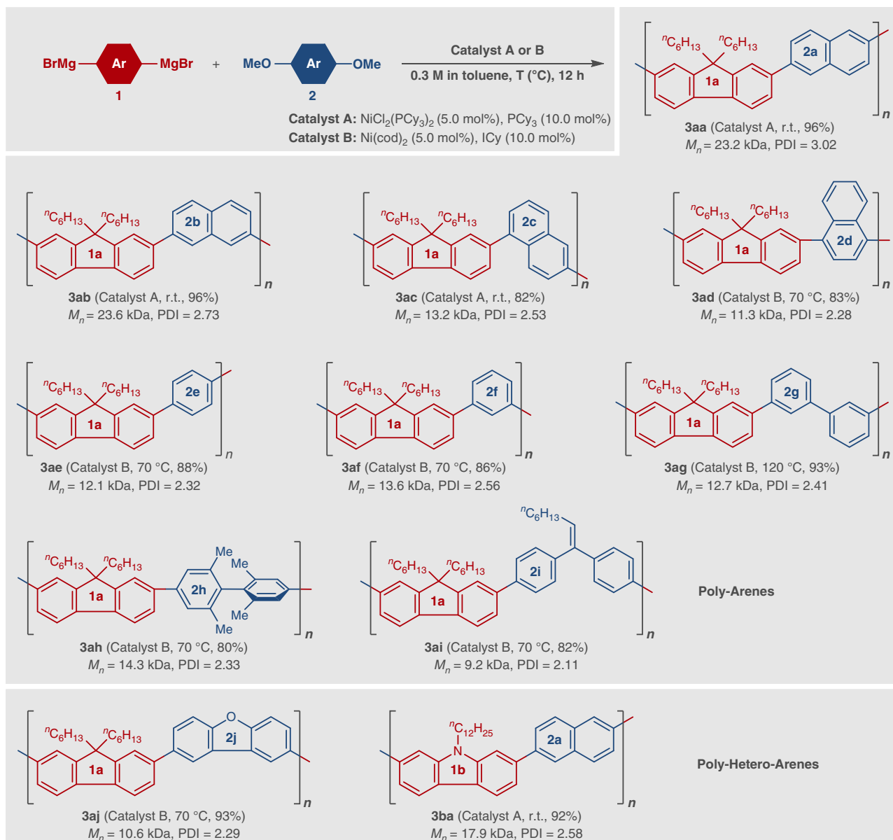
Fig. 2 Reaction Scope (1). Ni-catalyzed cross-coupling polycondensation between Grignard reagents 1 and dimethoxyarenes 2
