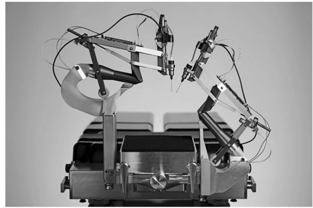
Fig. 4 The Preceyes Surgical System. An intraocular surgical system developed by Preceyes B.V [13].
