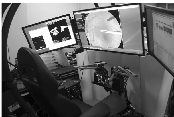
Fig. 8 The Future of Intraocular Robotic Surgery. Surgical cockpit enabled with augmented reality for robot-assisted, vitreoretinal surgery located in the Advanced Robotic Eye Surgery Lab at the University of California, Los Angeles.
