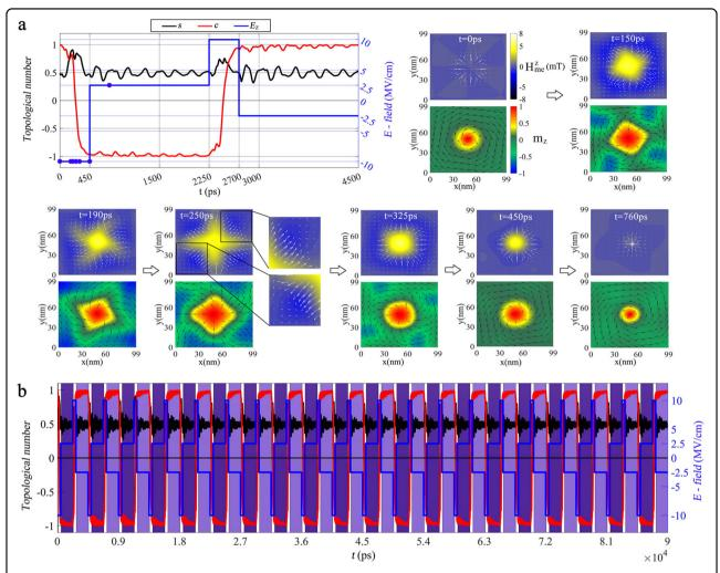
**Fig. 3 Vortex chirality reversal. a** Time evolution of the skyrmion and chirality numbers driven by the Gaussian pulse (k = 1) sequences with opposite field directions. Snapshot images illustrating the in-plane ME field (above) and magnetization configuration (below) at different stages of the vortex dynamics. **b** Reliable chirality switching between stable vortex states I (s = 1/2 and c = 1) and III (s = 1/2 and c = -1) by the same HCPs as in **a**.
