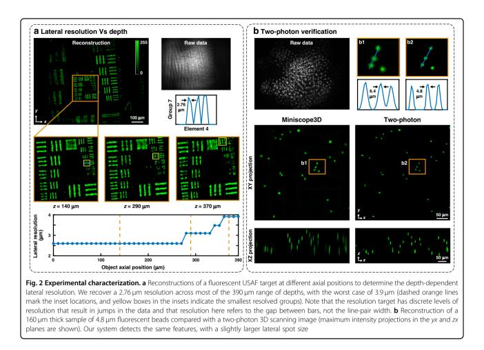
2.5 grams and achieves  $2.76 \,\mu\text{m}$  lateral and  $15 \,\mu\text{m}$  axial resolution across most of the  $900 \times 700 \times 390 \,\mu\text{m}^3$  volume at 40 volumes per second.
