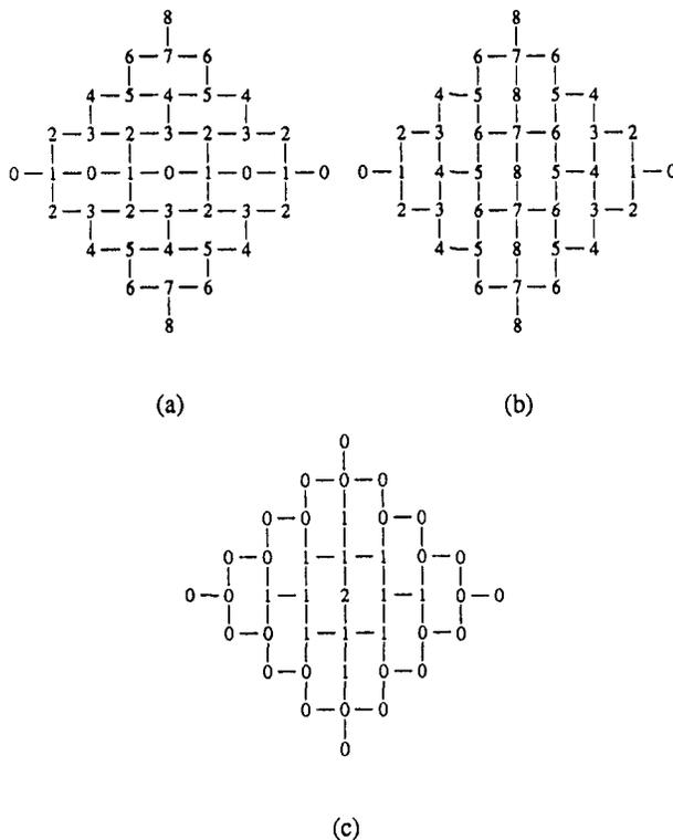
Fig. 5. Height functions of the all-horizontals and all-verticals tilings.
