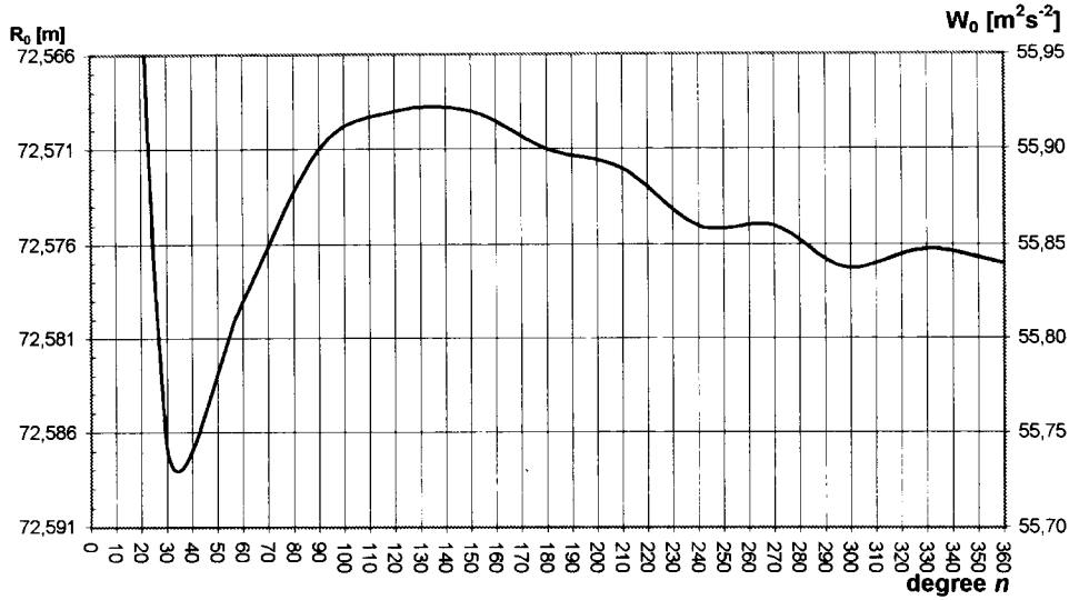
Figure 1. Dependence of W_0 ( 62\,636\,800\text{ m}^2\text{ s}^{-2} subtracted) and R_0 ( 6\,363\,600\text{ m} subtracted) on degree n of harmonics retained; geopotential model EGM96.
