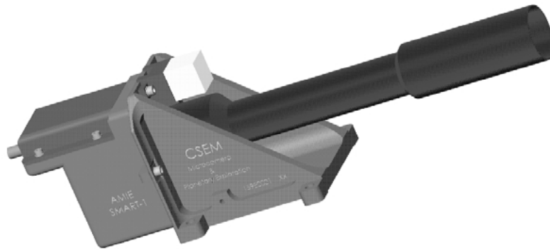
Figure 4. CAD view of the AMIE micro-imager head. The long tele-objective tube with the sun-baffle is fixed to the mounting frame. The cube of the proximity electronic is within the radiation shield shown at the left hand side.
