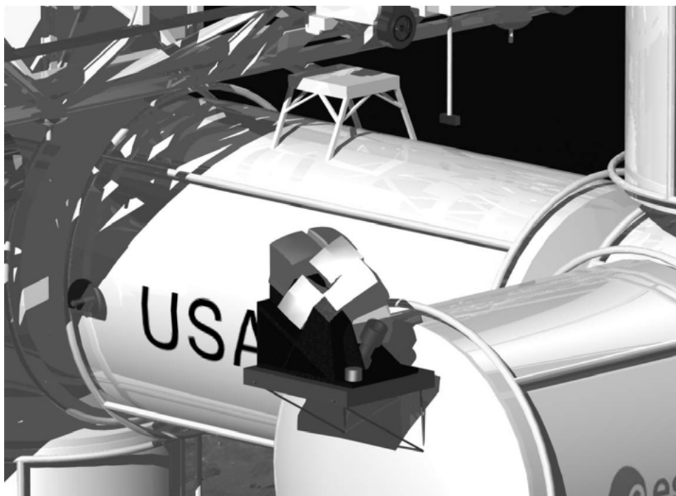
Figure 2. The proposed location of Lobster-ISS on the zenith pointing platform of the Columbus External Payload Facility.
