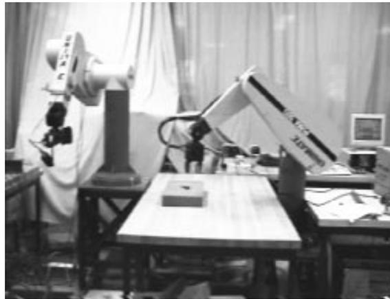
Figure 3. The experimental system, (a) consisting of the perceptual robot (left) and the grasping robot (right). The perceptual robot first scans the unknown object to yield a range image. A set of parameters is found which best fits the range data and this is used as a perception input to the learning system. The grasper then attempts to pick up the object based on the percept plus its acquired knowledge about the effectiveness of different grasp approach directions.
