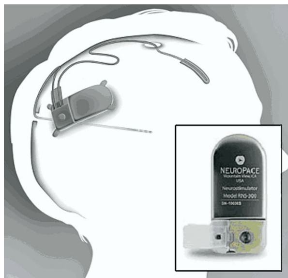
FIG. 2. Schematic of the NeuroPace RNS neurostimulator, depth and strip leads. Inset shows RNS neurostimulator.
