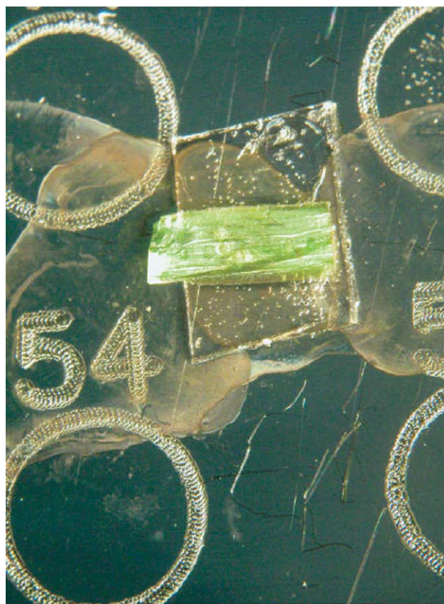
Figure 1. Stem tissue of Arabidopsis thaliana on a MALDI target plate. Sample was covered with colloidal silver for mass-spectrometric analysis.
