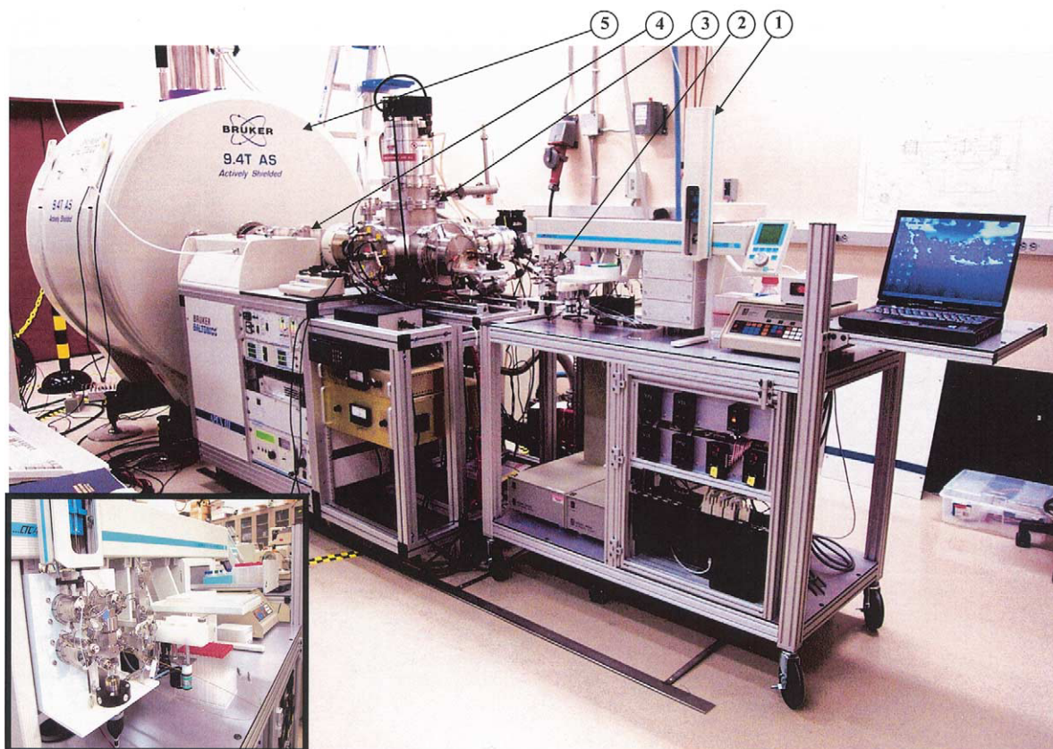
Figure 1. Photograph of the automated LC-FTICR instrument incorporating a 9.4 tesla superconducting magnet. Depicted in this photograph are: (1) The PAL autosampler, (2) the capillary LC system with injection valves, (3) the new front-end interface, (4) the commercial electrostatic ion guide, (5) the magnet. The Inset demonstrates injector valves and dual-capillary LC system.
