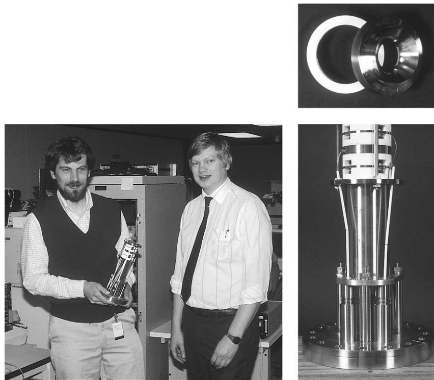
Figure 3. First research quadrupole ion trap analyzer designed and fabricated at Thermo Finnigan. The ring electrode is shown at the top with a corresponding alumina insulator. The radius ( r_0 ) of the hyperbolic surface was approximately 1 cm for this ring electrode. The photographs were taken circa 1984; John E. P. Syka is to the left and I am to the right in the figure.
