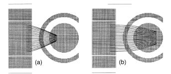
Figure 3. (a) Simion simulation of 100 eV ions exiting the 2-D trap along the length of the exit slot and being focussed onto the -15kV conversion dynode. (b) 10 keV ions simulated.
