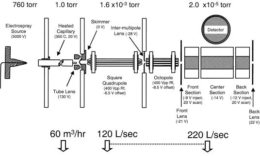
**Figure 5**. The overall instrument configuration along with typical operating voltages and pressures.
