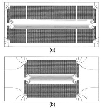
**Figure 2.** Simion simulation of the resonance excitation field comparing (**a**) a three section device and (**b**) a single section device with end plates for axial trapping.
