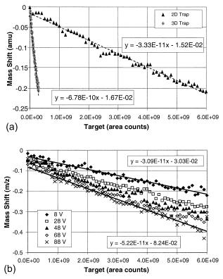
**Figure 6**. (a) Spectral space charge limit comparison between 2-D and 3-D ion traps. (b) The effect of the axial trapping potential on the spectral space charge limit for the 2-D trap.
