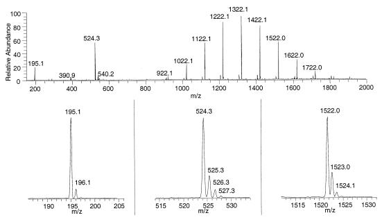
**Figure 8.** Full scan mass spectrum of the calibration mixture containing caffeine (m/z 195), the peptide MRFA (m/z 524), and Ultramark 1621 acquired at 5555 Da/sec with a 3  $\times$  10<sup>9</sup> target TIC.
