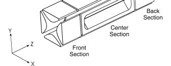
Figure 1. Basic design of the two-dimensional linear ion trap.
