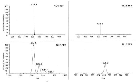
**Figure 10**. Isolation of  ${}^{13}$ C isotope of peptide MRFA at m/z 525.3 with high efficiency.
