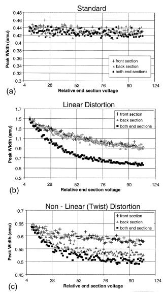
**Figure 7**. Effect of axial trapping potential on peak width for Ultramark at m/z 1522 for (**a**) a standard trap, (**b**) a linearly-distorted trap by slanting a rod, and (**c**) a non-linearly distorted trap by twisting a rod. Sections not scanned are held at 3 V relative to the center section.
