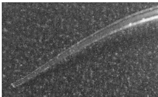
Figure 3. Microphotograph of the nebulizer tip. The bent shape, clearly visible in the picture, points the aerosol jet at the vaporization surface. The restricted orifice of the tip increases the liquid linear velocity and eases the aerosol formation under vacuum conditions.
