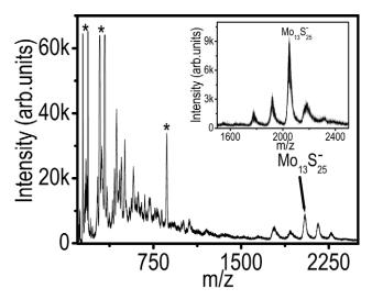
**Figure 4.** MALDI mass spectrum of the synthesized  $MoS_2$  nanoflakes with CHCA matrix in the negative ion mode showing the magic clusters. Lower mass range showing matrix-related peaks along with smaller clusters. The peaks marked with asterisks (\*) are attributed to the matrix. Inset shows the MALDI mass spectrum of synthesized  $MoS_2$  nanoflakes with IAA matrix in the region of interest.
