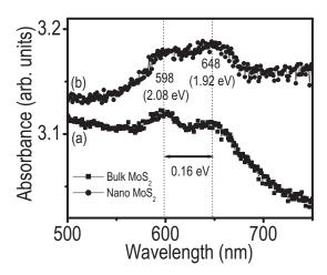
**Figure 1.** UV-visible diffused reflectance spectra of bulk  $MoS_2$  (a) and synthesized  $MoS_2$  (b).
