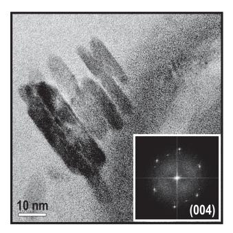
Figure 2. HRTEM image of the synthesized nano MoS<sub>2</sub> flakes. Stacked nanoflakes are seen. Inset: Fourier transform of the image showing a hexagonal pattern.
