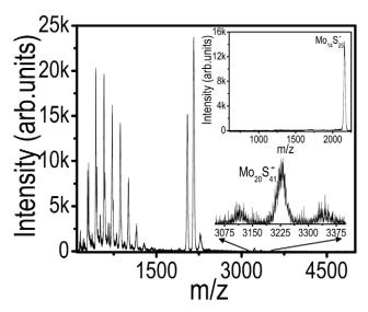
Figure 6. LDI mass spectrum of derived MoS<sub>2</sub> nanoflakes after UV irradiation in the negative mode showing the magic number cage clusters. A weak peak attributed to a Mo<sub>20</sub> cluster is also shown. Enlarged peak of Mo<sub>20</sub>S<sub>41</sub> is also shown, above the spectrum. Inset: PSD mode LDI mass spectrum of  $\mathrm{Mo}_{14}\mathrm{S}_{25}^{-}$ showing no fragmentation. The PSD data were collected in four separate regions and stitched together later.
