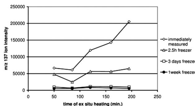
**Figure 2.** Ion intensities of  $m/z$  137 from samples of gold-coated DHBPh in polyvinylbutyral, ex situ heated at 40 °C for a period between 50 and 200 min and immediately measured or stored up to 1 wk at –8 °C as a function of time
