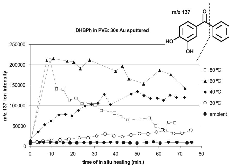
**Figure 1.** Ion intensities of  $m/z$  137 from samples of gold-coated DHBPh in PVB, heated in situ (i.e., inside the S-SIMS analysis chamber) at 30, 40, 60, and 80 °C as a function of the heating time.
